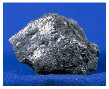
Graphite is an excellent conductor of heat and electricity. It has the highest natural strength and stiffness of any material; it maintains its strength and stability to temperatures in excess of 3,600 °C. It is one of the lightest of all reinforcing agents. It also has high natural lubricity, and is chemically inert with a high resistance to corrosion.
